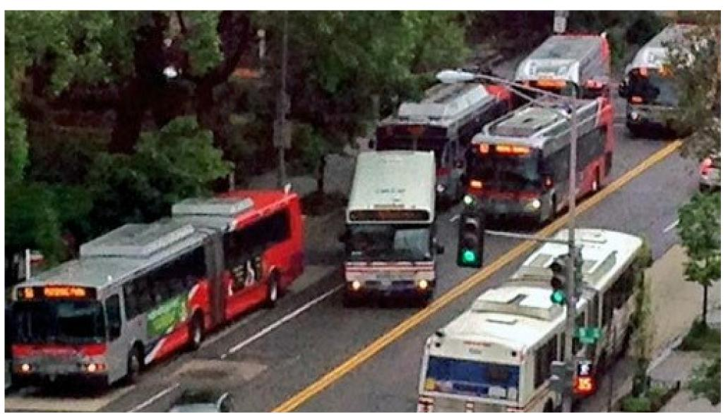
Stop bypass and real-time information for boarding passengers at a stop to be skipped can aid in increasing vehicle separation.
